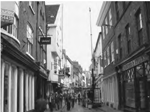
Figure 5.1c Telescopic mast-mounted camera used to record high-level fabric in a restricted urban setting (Credit: Aerial Viewpoint).
